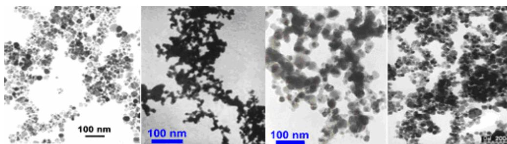
Figure 1: Purchased nanopowders from left to right: Fe<sub>3</sub>O<sub>4</sub> (SkySprings Nano), Cu (NanoAmor), Cu-C (NanoAmor), Fe<sub>3</sub>O<sub>4</sub> – PVP (NanoAmor)
