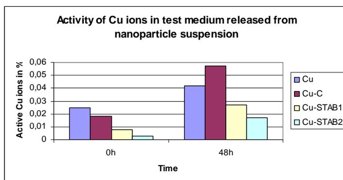
**Figure 3:** Copper ion activity of 4 different CuNP was measured using a copper selective electrode. By means of a standard regression line the measured potentials of the electrode was transformed into concentrations and are represented as percentage of the nominal concentration of the particle suspension. The activity can be regarded as the quantitative indication for the amounts of free and unbound copper ions in solution.
