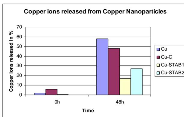
**Figure 2:** Copper ions released from 4 NPs with different surface modifications were quantified in the supernatant after centrifugation using flame and graphite furnace atomic absorption spectroscopy. Total amounts of copper were also quantified by flame AAS using the same initial concentration as for the ion release measurement but excluding the centrifugation step. The quantified released ions are represented in percentage of the total analytical amounts.
