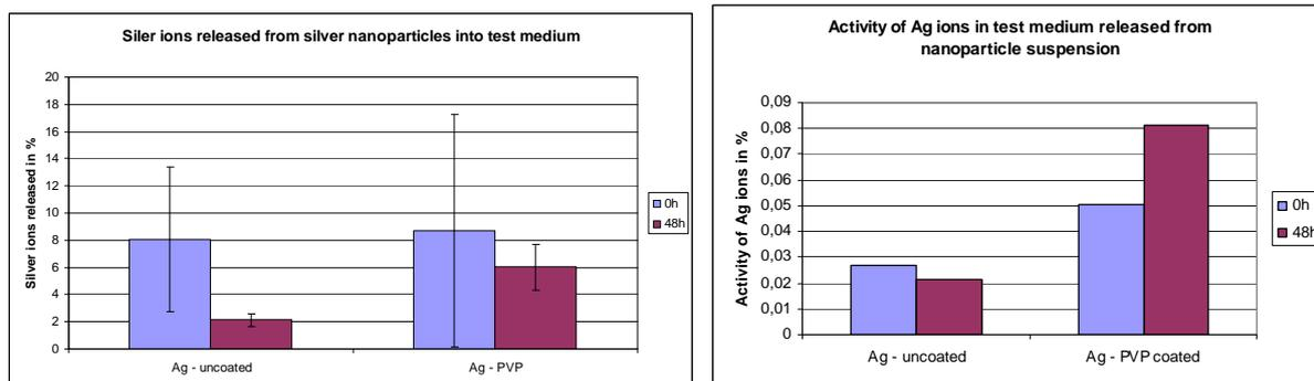
**Figure 7:** Left: Ag ion release from coated and uncoated AgNP dispersions as determined by AAS. Right: Determination of Ag ion activity in coated and uncoated AgNP dispersions.
