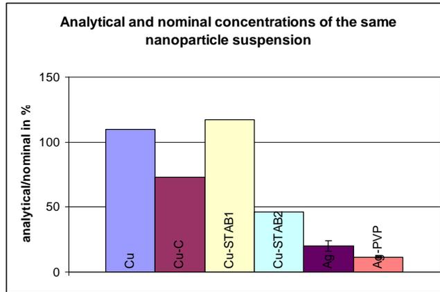
**Figure 10:** Comparison of analytical NP concentrations in percentage of nominal concentrations for 4 Cu NPs and 2 Ag NPs in test medium after 48h. No replicates were performed for the 4 CuNPs and a total of 3 replicates were performed for the 2 AgNPs.
