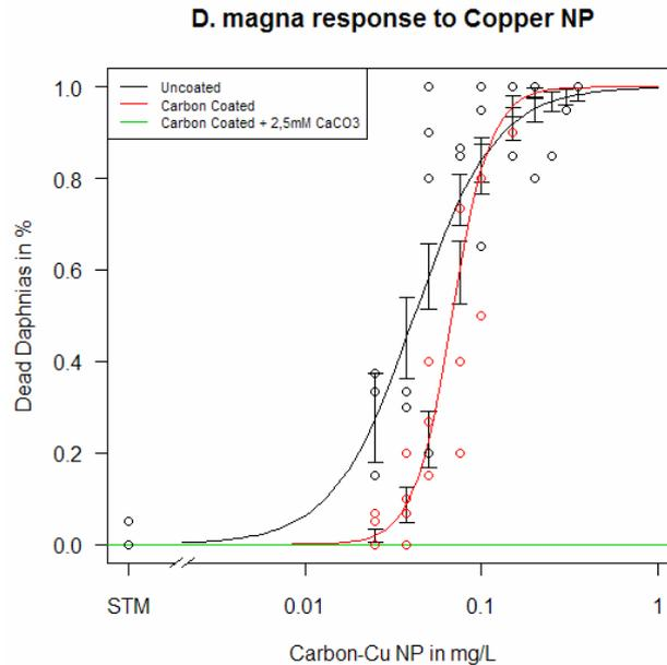
**Figure 8:** Dose response curve of 48h exposure of carbon coated and non-coated copper NPs to *D. magna*. Non-coated copper particles are more toxic than carbon coated particles and the addition of 2,5mM CaCO<sub>3</sub> drastically reduces the toxic effects of carbon coated copper particles.
