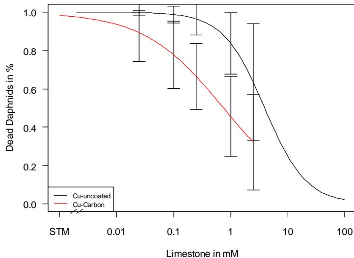
**Figure 9:** D. magna exposure tests with constant 0,2mg/L C-CuNP and CuNP but increasing concentrations of CaCO<sub>3</sub>. Toxicity mitigating effects with increasing concentrations of CaCO<sub>3</sub> can be observed.
