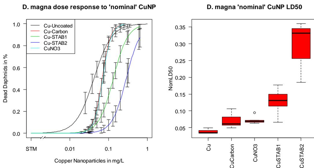
**Figure 1:** Left: Dose response curves for 4 NPs and a copper reference, using nominal exposure concentrations. Right: Boxplots of LD50 values where the red box is the interquartile range, thick black line is the median and the whiskers are standard error. LD50 values calculated individually for every replicate of each particle or reference.
