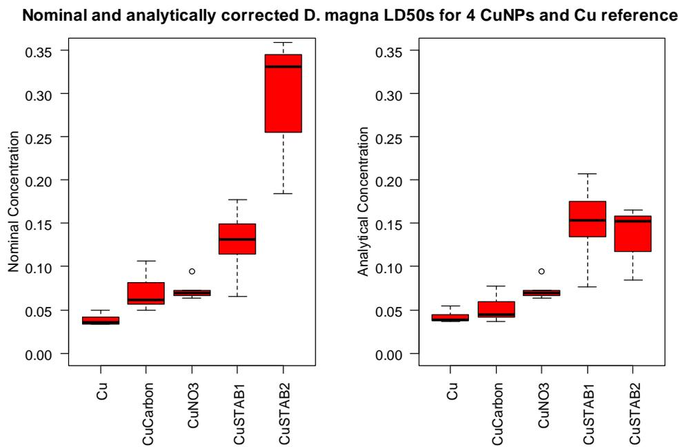
**Figure 11:** AAS was performed on all copper particles after 0h and 48h for two different concentrations. Those results were used to correct the exposure concentrations during biological response tests. All concentration are given in mg/L.
